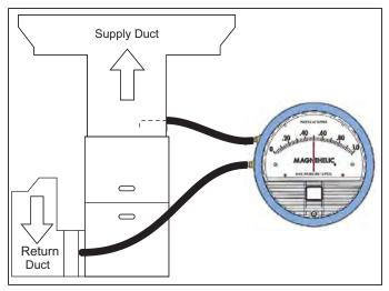
Set appropriate airflow per temperature rise for gas heating. Set appropriate airflow per "Blower Performance CFM" table for cooling/heat pump heating operating based on outdoor unit size.
